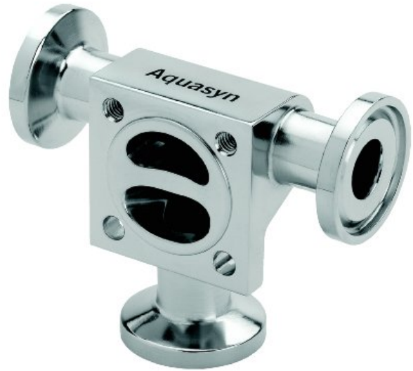
ZERO-STATIC TEE BODY • MACHINED FROM A SINGLE BLOCK • AQUASYN ARCHIVE
